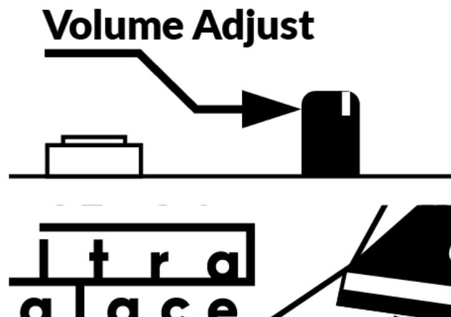
Adjust the volume of the Audio Click. Rotate clockwise for louder and counter-clockwise for quieter or silent.
