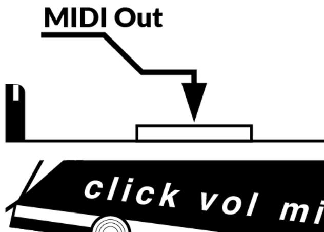
This is the MIDI OUT, to be connected to the MIDI IN on another device. This will send MIDI clock and MIDI commands. MIDI THRU and MIDI OUT can be used on the other device to daisy chain this signal. MIDI splitters and converters can also be used.
