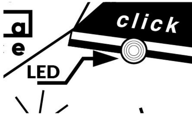
The LED will flash while the MIDINOME is **Active**, it will flash in sync with the MIDI signal and the audio click or CV clock.
