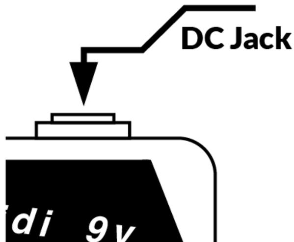
Midinome takes a standard 2.1 mm power jack, 9VDC. As is common with guitar pedals, it is **centre negative** to fit easily on your pedalboard. Midinome is reverse polarity protected, so no worries if the wrong type of adapter gets plugged in.
