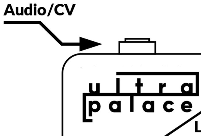
This 3.5 mm stereo or mono output carries the Audio Click or CV Clock, perfect for headphones or Eurorack patch cables. This output is powerful enough to drive headphones, and the volume control can be used to adjust for line level, suitable for mixers, audio interfaces, or other line level equipment.
