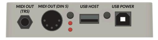
To power Midithrone, use a USB-B cable to connect to any 5V USB power supply, such as a phone charger or other USB power source. A USB battery bank can also work well.
